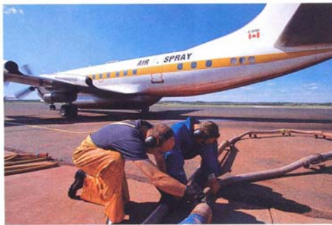
A ground crew prepares to refill an L-188 Electra air tanker with fire retardant.
